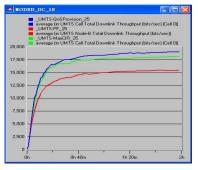
• Figure 7. Cell throughput comparison
