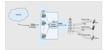
Figure 2. The HSDPA Packet Scheduler Model 2.3. Packet Scheduling Algorithm in HSDPA
