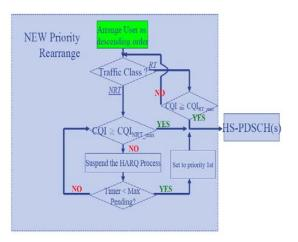
Figure 4. Flow Chart of normal condition scheduling
